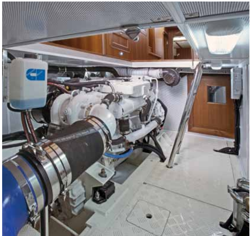
ABOVE This single Cummins MerCruiser 380 hp diesel offers modest speeds, but good fuel efficiency.
