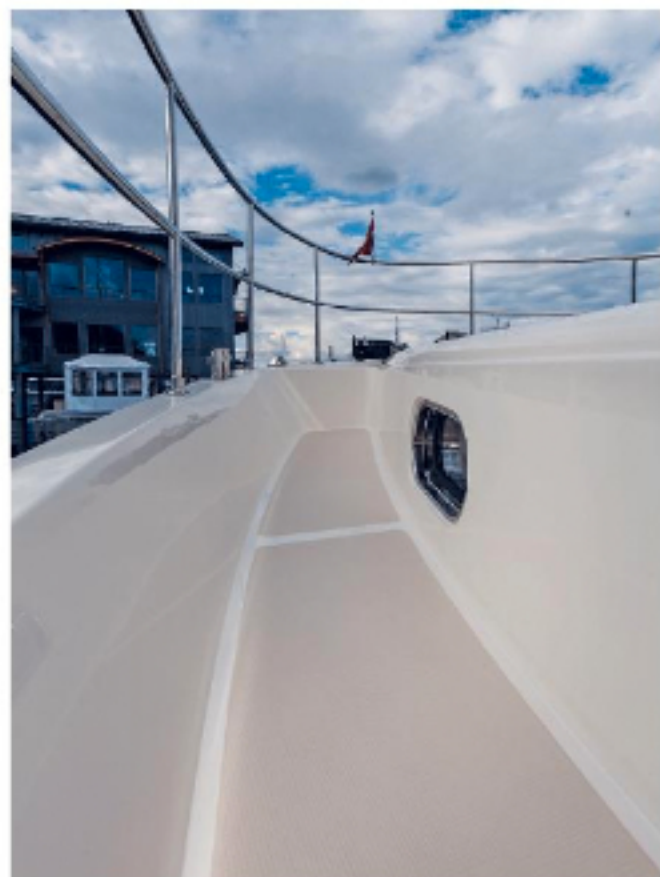
BULWARKS CONTINUE ON BOTH SIDES OF FOREDECK, UNTIL ONLY A STEP OR TWO AWAY FROM THE BOW.
