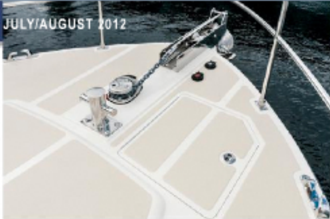
ABOVE: SELF TAILING WINDLASS AND SAMSON POST HELP MANAGE GROUND TACKLE.
