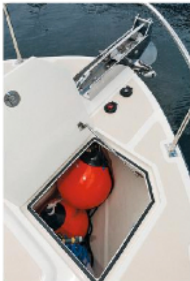
ABOVE: SELF TAILING WINDLASS AND SAMSON POST HELP MANAGE GROUND TACKLE.
